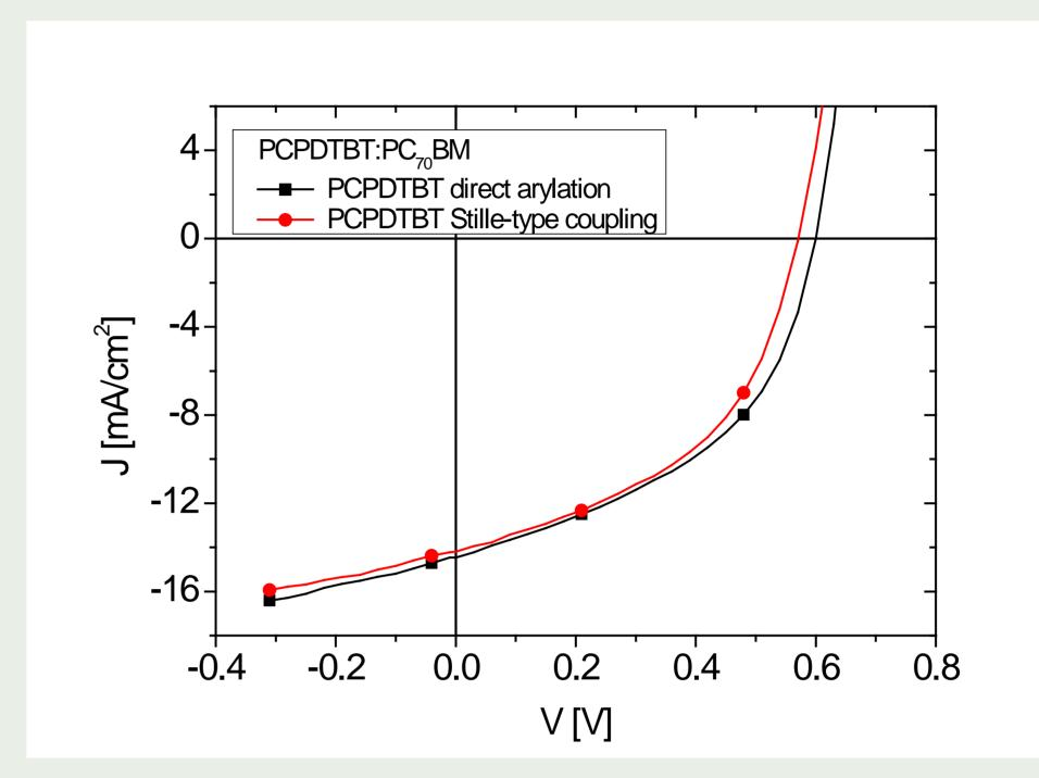
I/V-characteristics of inverted OSCs with PCPDTBT as donor and PC<sub>70</sub>BM as acceptor (solvent: chlorobenzene, processing additive: octane-1,8-dithiol).
