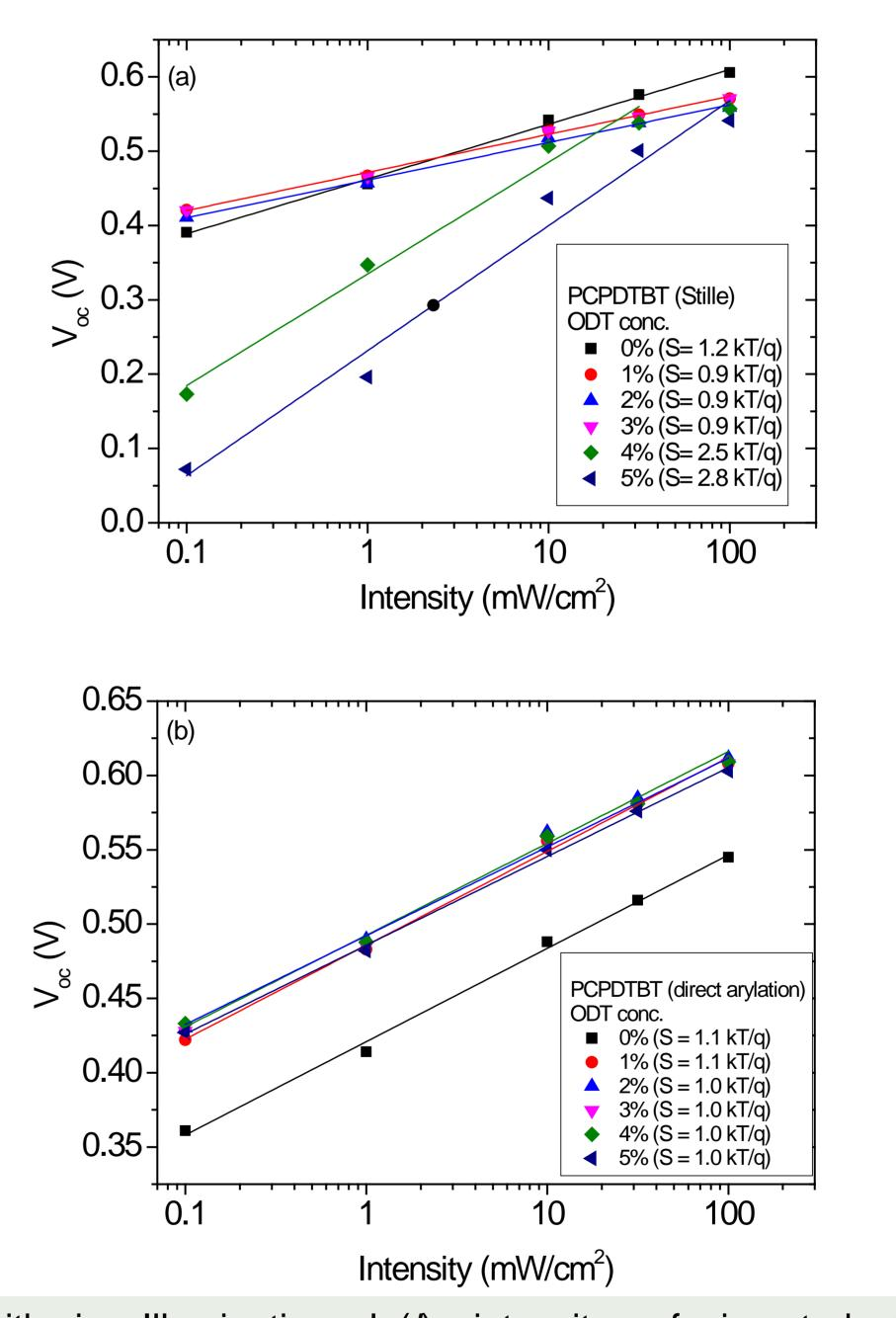
vs. logarithmic Illumination In(I) intensity of inverted OSCs based on PCPDTBT/PC<sub>70</sub>BM prepared by (a) Stille-type coupling and (b) by DAP. The slope S of  $V_{oc}$  vs. ln(I) is close to kT/q indicating the absence of trap assited recombination due to impurities or defects.<sup>[2-4]</sup> Only for increased amounts of processing additive ODT OSCs based on Stille-type PCPDTBT show an increased S value.
